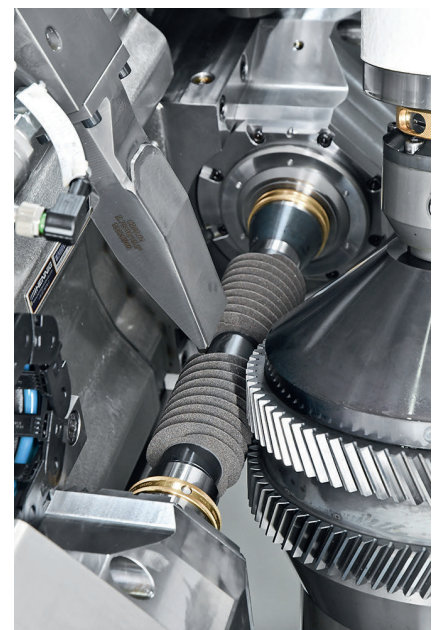
2 Robuste, abrichtbare CBN-Schleifscheibe © Liebherr
